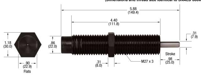
The SNALD 600MH-563 is the popular choice for mold housing installations. This dependable model is used on series 1 & 2 type 1 mold housings and some stretch rod applications where no shock holder is used. If a softer stiffness is desired consider using the SNALD 600M-562. Dimensions and thread size are identical.
