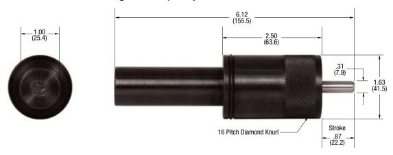
The SNALD 600-574-QCM model provides an integral built-in shock holder with SNALD 600M-562-ERSB technology. This QUICK CHANGE shock absorber for series 2 stretch rods eliminates assembly issues associated with re-used shock holder thread quality.
