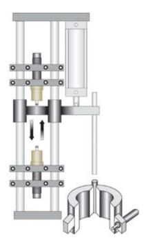
On this machine version the mechanical cam has been eliminated and only the air cylinder is used to operate the stretch rod slide. The cylinder body is stationary and the piston rod moves the slide up and down.
