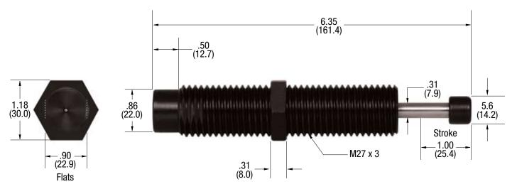
Base model installations with lock nut...position the shock absorber to use 7/8" (22 mm) of stroke. Rod projection with button is 1.47" (37.3 mm). Do not install the shock absorber to use more than 7/8" (22 mm) of stroke.
